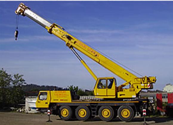
A yellow mobile crane with a telescopic boom, parked on a paved area under a clear blue sky. The crane is mounted on a multi-axle truck chassis.                                              |
